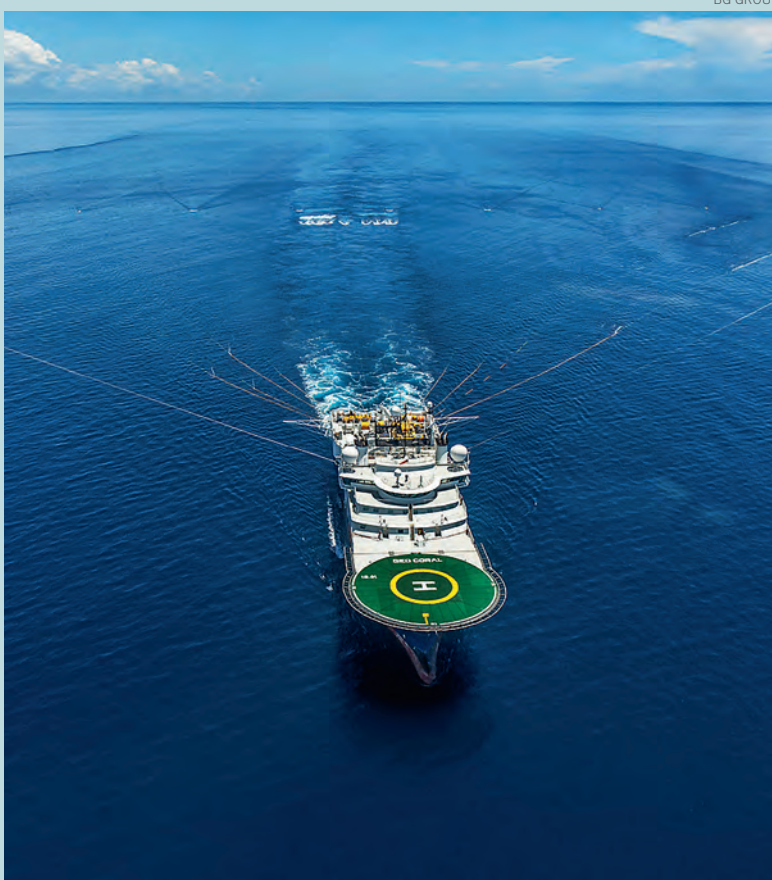
BG Group used survey vessel MV Geo Coral to gather seismic data off the coast of Tanzania in 2013
