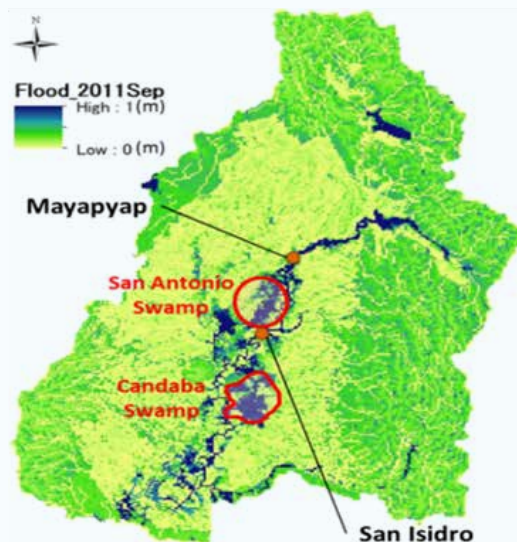
Figure 7.3.2 Results from inundation analysis of the Pampanga river basin by using the RRI model. Map © ICHARM
