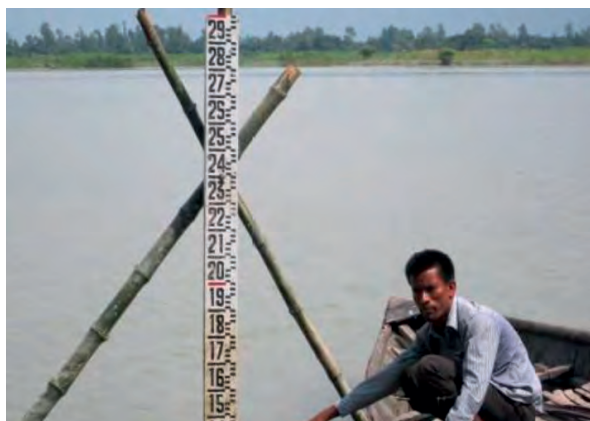
Figure 2: Typical water level gauge in the River (Source: FFWC)
