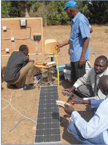
Sizing of a solar system and simulation of an electric breakdown during practical training organized as part of the African solar summer school, 2010
