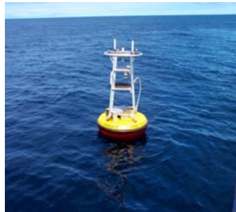
Chilean ocean drifter used in tsunami early warning system (2005, Shoa © UNESCO)
