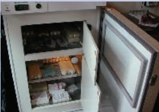
Solar-powered refrigerator used to conserve vaccines in health-care centres in rural and isolated areas. This technology was one of the subjects of this year's solar school
