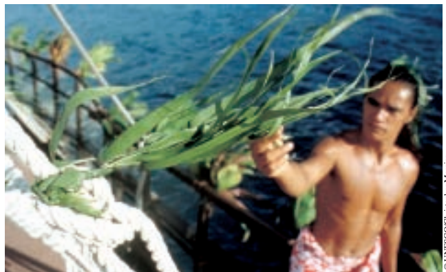
Traditional navigation in the Pacific; foliage in the boat rigging provides a simple means of following subtle changes in the direction and strength of the wind
