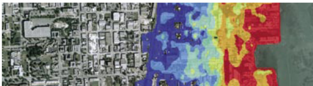
Fig. 4.6 Inundation modelling of a storm surge impact. This model simulated a Category 5 hurricane generating a surge height of 7 m impacting Miami, U.S.A. The colour scale is based on modelled inundation depths: Blue = <1 m; Green = <2 m; Yellow = <3 m; Orange = <4 m; Red = >4 m. Atlantic Ocean to Right of image. Source: Courtesy Ambiental Technical Solutions, Ltd. ( www.ambiental.co.uk ).
