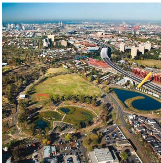
Our cities are water supply catchments – as illustrated by the Royal Park Wetland in Melbourne, used for harvesting and treating urban stormwater
