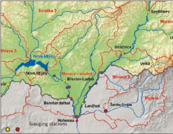
The above detail shows: sub-basin borders (red lines); water gauges operated by CHMI (yellow), Povodí Moravy (orange), SHMI and Lower Austria hydrology department (red); and new monitoring sites operated by Morava River Authority (purple)
