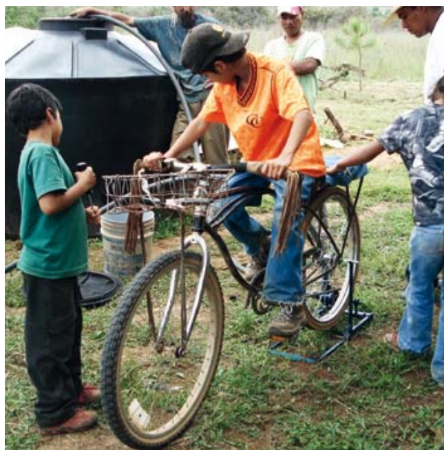
A bicycle adapted as a pedal-powered pump for irrigation purposes in the community of San Pedro, Pátzcuaro
