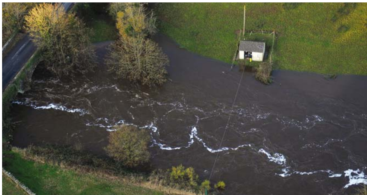
River flow gauging on the River Blackwater in Northern Ireland during a flood event in November 2009
