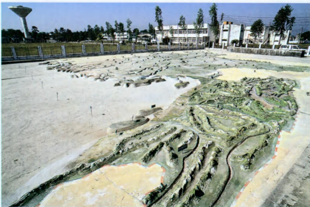
This model at a research centre in Faridpur (Bangladesh) is used to study flood patterns. The results will be helpful in designing and building flood-control barrages.
