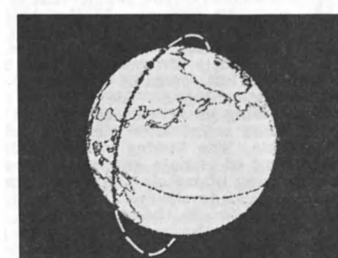
SATELLITE'S ORBIT brings it over a different part of the globe (due to earth's rotation) on each of its completed circles. Its orbit is so steady and it has lost so little speed that its path in relation to the earth can easily be computed in advance. These five diagrams show different orbits, the first being the one taking the "man-made moon" over Moscow.
