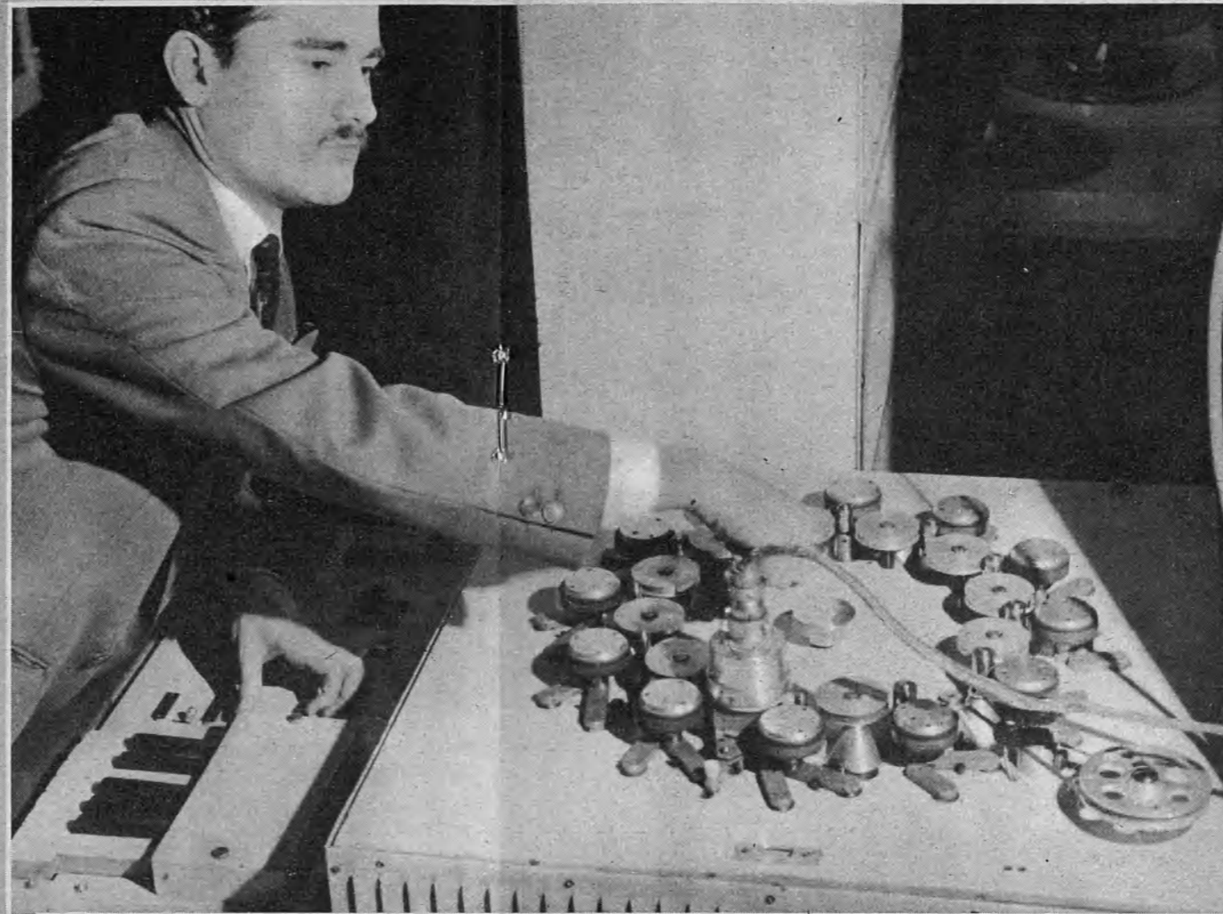
PRESTIDIGITATOR: This instrument makes it possible to modify the form of tape-recorded sound by changing the speeds, thus raising or lowering the pitch of the original sound and greatly altering its tone quality. Even more radical changes can be brought about by reversing the tape in the machine.
