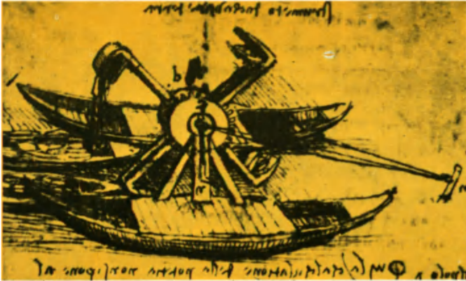
Leonardo sketched this dredger resembling a twin-hulled catamaran. "This plough will be able to dislodge the mud from the bottom," he wrote, "and unload it upon the barge which is placed underneath it."
