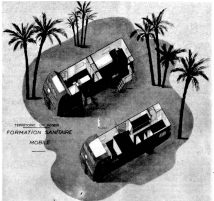
This overhead drawing shows the two trucks of the medical team which will shortly go into action in the most isolated parts of French Nigeria. The medical truck (on left) houses the doctor's office and X-ray camera, with an operating table for emergency cases. The second truck has housing facilities "easily comparable with those found in many small homes".
