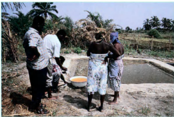
Below, salt is produced from brine by solar evaporation at the village of Kpablé (Benin). Bottom, pans of brine are heated on wood stoves.
