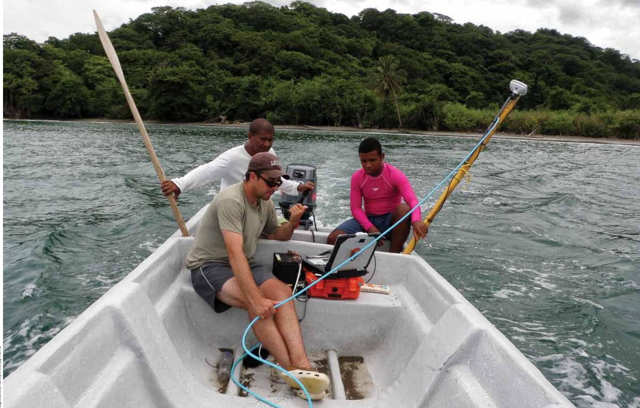
Magnetometer survey in the bay © B. Ho
