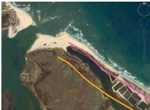
Model prediction of coastline change by 2100 at Tu Hien inlet in Vietnam, where rainfall is projected to rise. Purple line: Bruun effect alone; yellow line: Bruun effect plus basin infilling; red line: Bruun effect, basin infilling plus the effects of rainfall and runoff combined.
