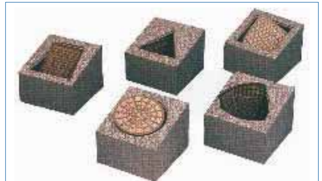
Ever wondered why manhole covers are round? A square cover can fall into a square manhole of the same size. This is because the diagonal of a square is longer than the length of its sides. Conversely, a round cover cannot fall into a round manhole of the same size because a circle is of constant width. In other words, the distance between any two parallel lines which are tangent to the circle is constant. Thus, there is no danger with a round manhole of its slipping into the bowels of the city sewers, perhaps taking a pedestrian with it...
