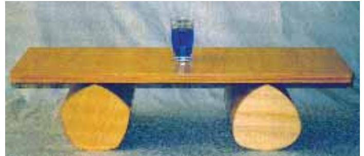
Need to move a heavy load? One method involves placing a board on top of two logs. The circular cross-sections of the logs allow these to roll smoothly. The same can be said for rollers whose cross-sections are other figures with constant width, as demonstrated by the non-circular logs above
