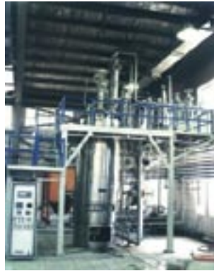
The 3000-litre fermenter used to produce B.t. M-H-14 . To form the toxin, the bacteria are cultivated in the fermenter with the culture media at a temperature of 30°C. It takes only 28 hours to form the toxin after inoculating the bacterium
