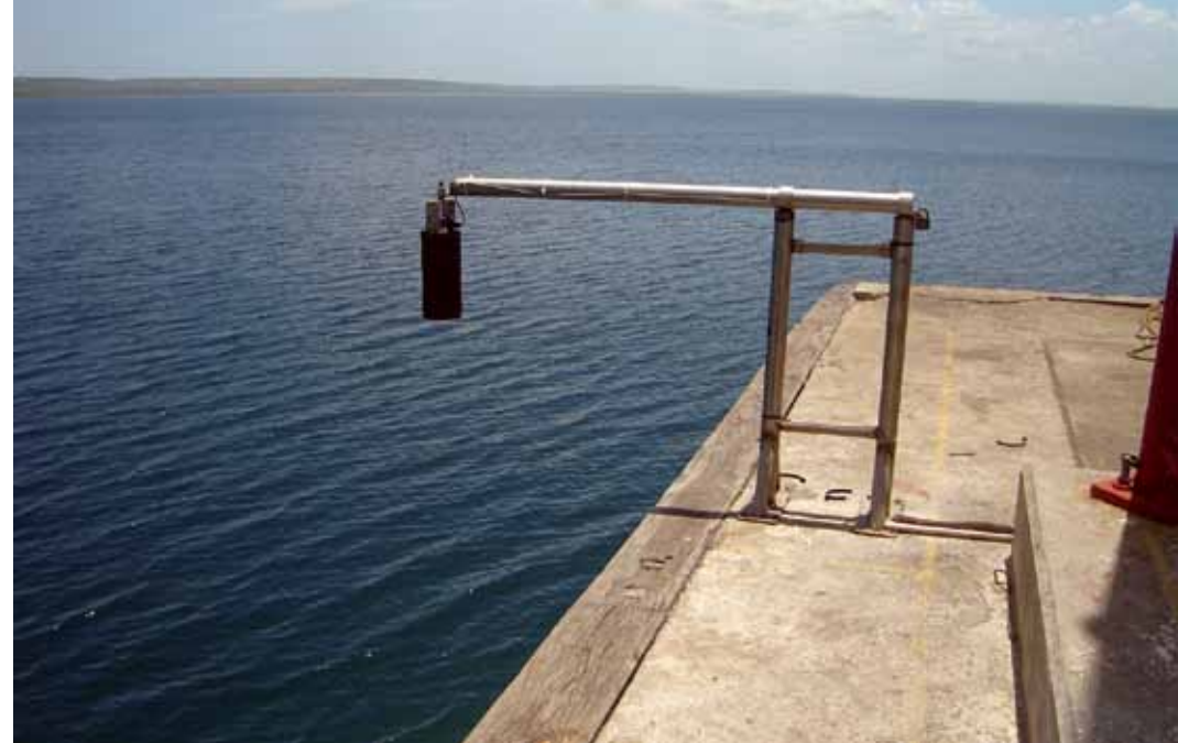
Figure 2. Tide gauge at Kalesto, Pemba Quay, 2006.
