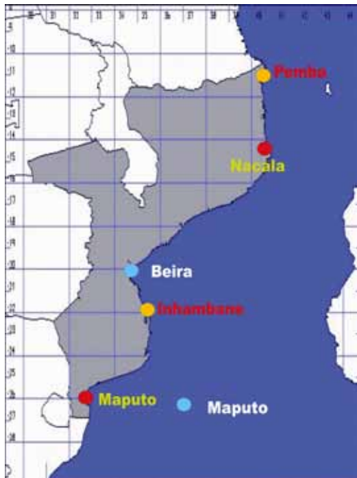
Figure 3. Installation of the various types of tide stations in Mozambique. Red indicates the locations where the OTT R20 tide type were installed; yellow is the locations where the radar tide gauges were installed (GLOSS stations), and blue is the stations where INAHINA installed the radar tide gauges.
