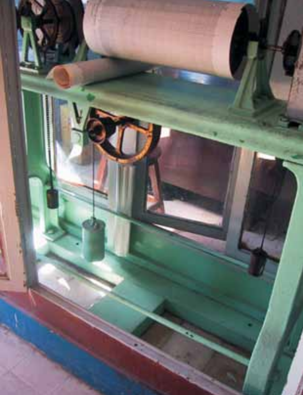
Figure 3. Old tide gauge at Alexandria Port.
