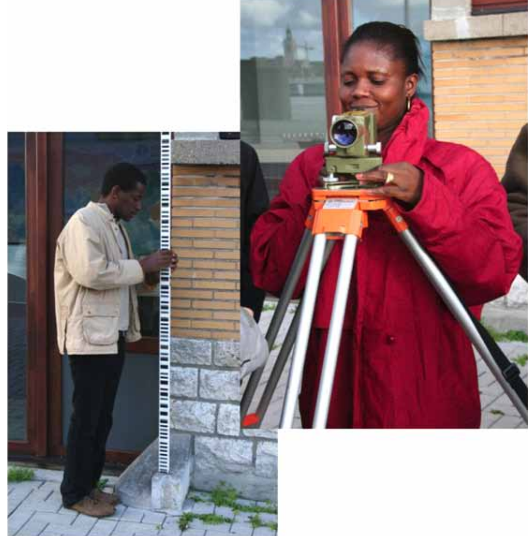
Figure 4. Technicians practice levelling of tide gauge benchmarks at a training course in Ostende, Belgium.
