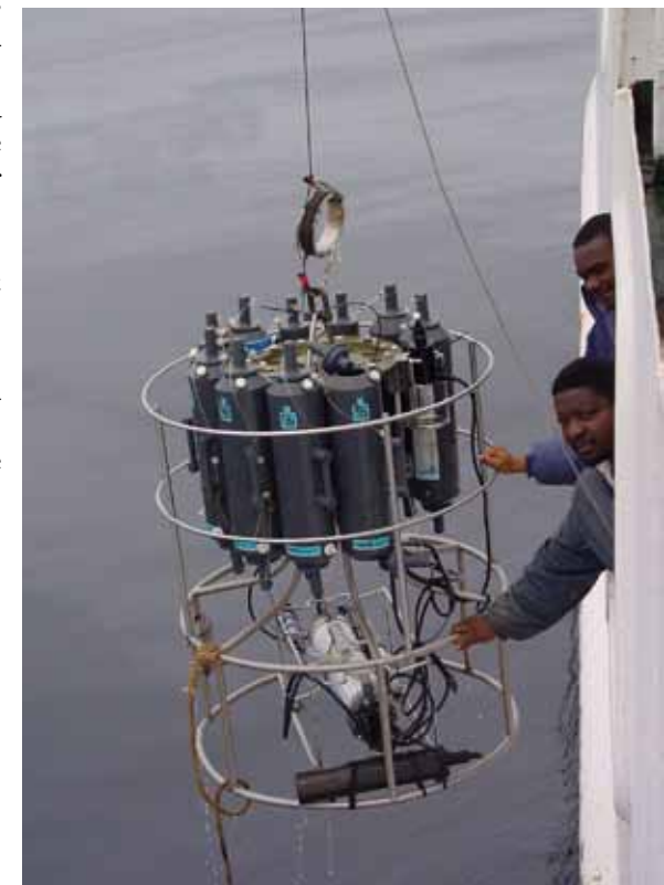
Figure 2. CTD which is used on the "R.V Welwitchia" for oceanographic measurements (photo taken by Deon Louw).
