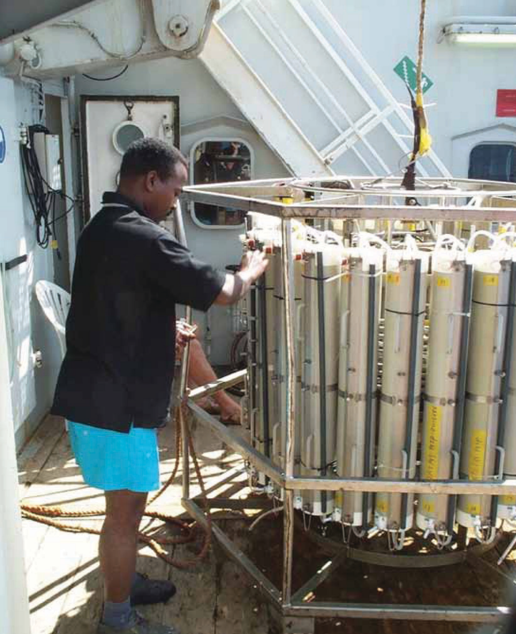
Figure 7. Scientist from Madagascar prepares sampling bottles for launch from a research vessel.
