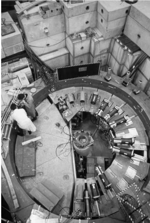
Plate 71 Nuclear particle accelerator at the European Organization for Nuclear Research (CERN), near Geneva, Switzerland. This instrument uses electric fields to propel charged particles to great energies (Photo © Marc Garanger).
