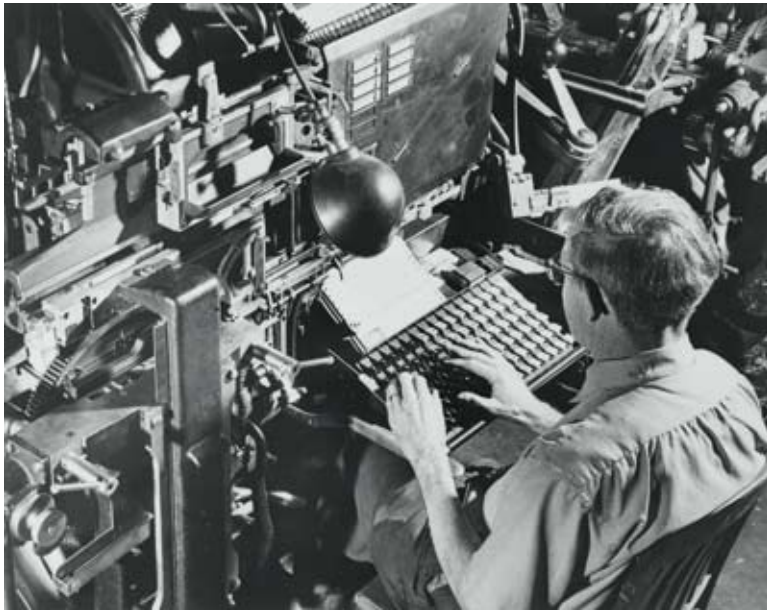
Plate 130 A typesetter working on a linotype machine, 1970. First produced in 1886, the linotype machine, with its ninety-character keyboard, transformed the printing industry (Photo © Bettmann/Corbis).
