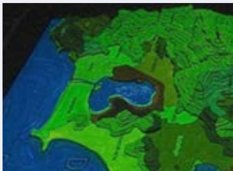
Figure 3: Projecting a district map (see above, in the middle) over our 3D model made of many slices of the coloured foam.
