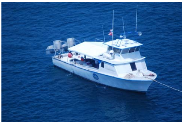
Figure 2.5.a. Top: The Blue Water Rose boat used by IMDI. The propeller deflectors used in the excavation of the site attributed to the San José wreck can be seen on the stern. © UNESCO
