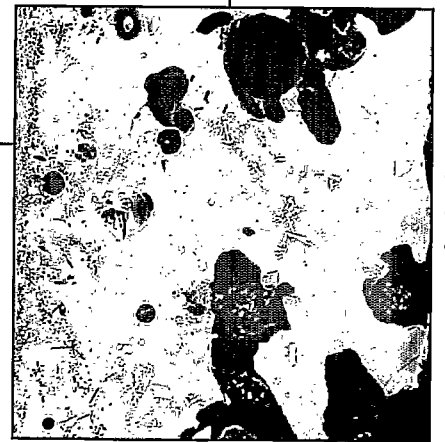
Back-scattered electron photomicrograph of pottery similar to the Basra bowl, showing glaze. Note the various inclusions, including round bubbles, dark quartz grains, thin wollastonite crystals, and white tin-oxide particles.
