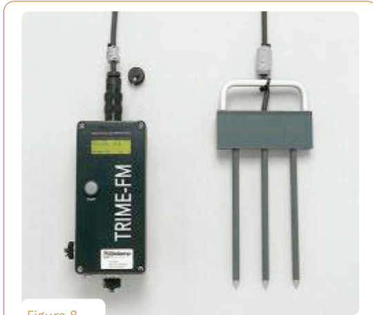
Figure 8. Trime-FM TDR (Eijkelkamp Agrisearch Equipment, Giesbeek). © M. Ouessar, M. Sghaier, M. De Boever, D. Gabriels
