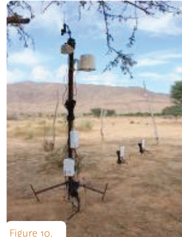
Figure 10. Installed weather station and TDR sensors under one tree inside National Park Bou Hedma © M. Ouessar, M. Sghaier, M. De Boever, D. Gabriels
