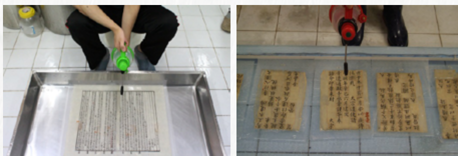
Wet cleaning, immersing relic in a tub Wet cleaning, spraying neutral water
