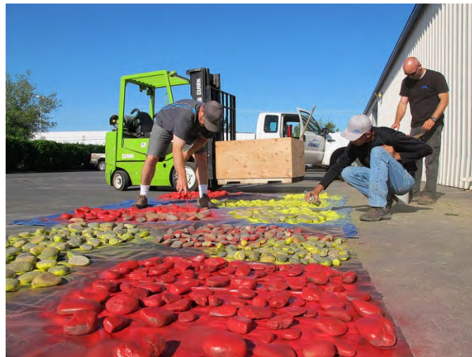
Figure 8: Colouring particles for tracking of river bed sediments
