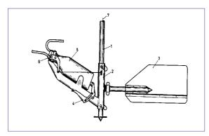
Figure 3. Water Sampler for suspended solids analysis.
