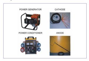
**Figure 5.** Electrofishing equipment (photo A. Bednarek).
