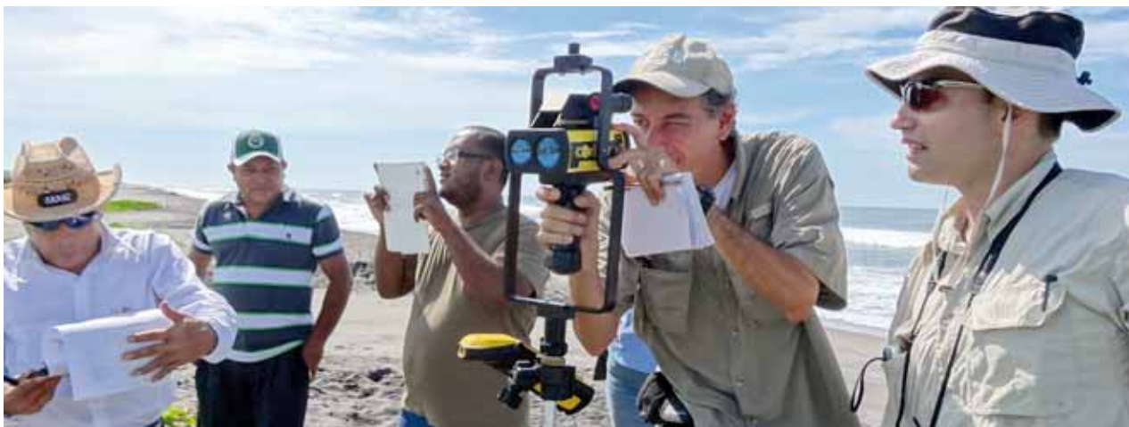
ITST measuring tsunami runup using laser rangefinder in El Salvador, 2012. Photo courtesy of ITIC
