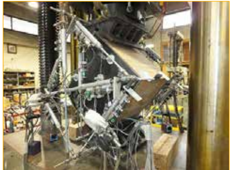
Figure 4.2.7. Anchoring of reinforcement (steel panel)
