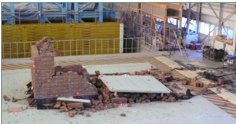
Figure 4.1.5. Model structure after shaking
