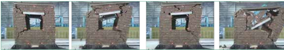
Figure 4.1.4. Process of specimen collapse in the shaking table test (Excitation number 10)
