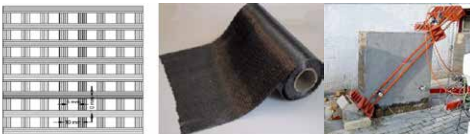
Figure 4.2.3. Fiber-Reinforced Cement Matrix (FRCM) [4.16]
