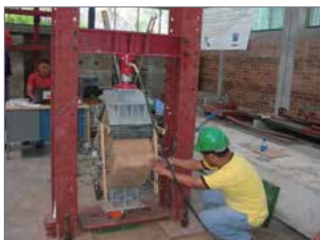
A.2.14 Seismic capacity experiment of a commonly used brick
