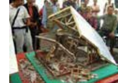
The final stage of the demonstration: The model house of poor construction totally collapsed.
