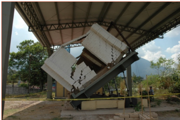
Figure 5.4.2 Very simple and effective experiment with full scale model using tilting table
