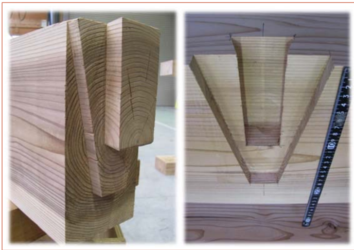
Figure 5.4.5 An example of pre-cut timber cut by numerical control cutting machines
