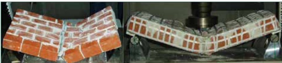
Figure 3. Out-of-plane test (brick) (unreinforced (left) and reinforced by pp-band (right))
