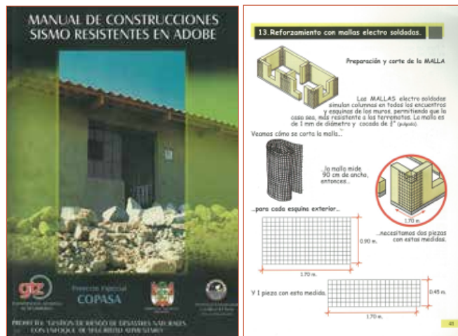
Figure 5.2.1 An example of technical guidelines (Manual for Earthquake Resistant Adobe Houses in Peru. Left: cover, right: an example of reinforcing with wire mesh)
