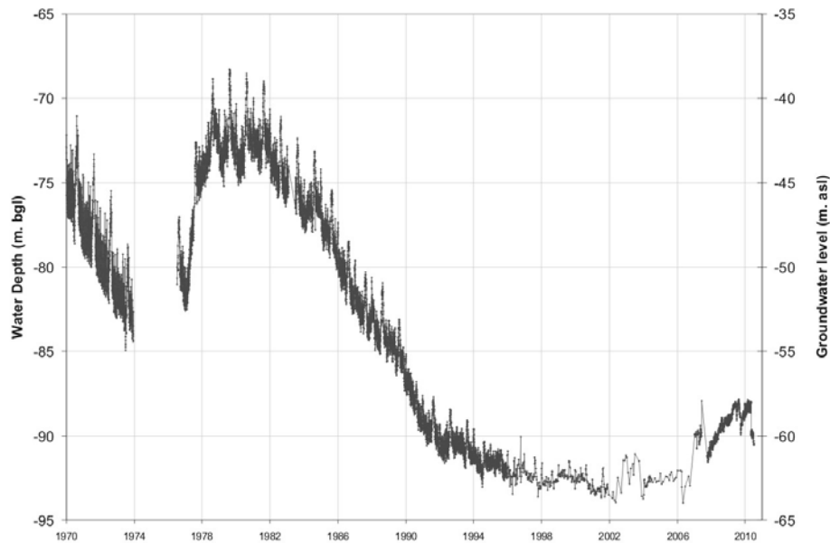
Figure 1: Piezometrical level (m) in a monitored borehole in Bondues (Fr), from 1970 to 2010.
