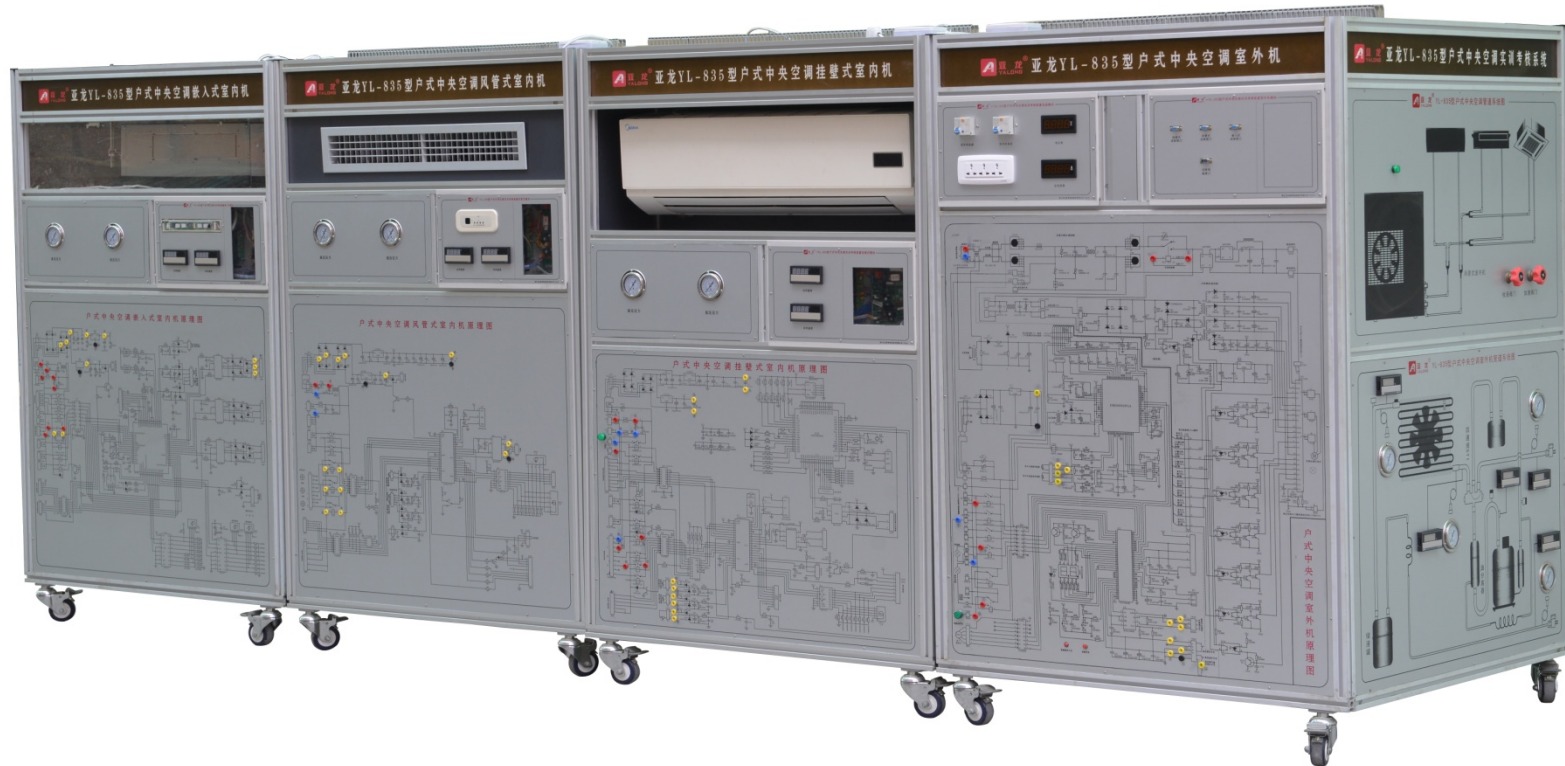
亚龙YL-835户式中央空调实训考核系统 YALONG YL-835 Household Central Air Conditioner Training and Assessment equipment
