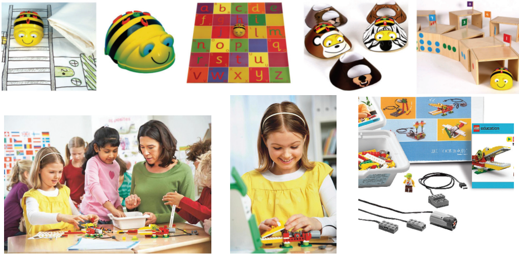
Figure 4.2.10 TTS programmable floor robot Bee-Bot with various mats, jungle jackets and tunnels ( www.tts-group.co.uk ). Other kinds of clip-on covers are available so that they can be easily transformed into different identities or programmable LEGO WeDo robots with different sensors to control its behaviour
