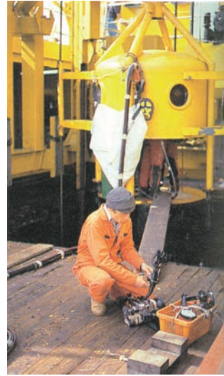
▲ © AAO. Open bell diving during a research project in the Netherlands North Sea sector. The aims of the project and its location define the type of diving. Open bell diving from a dynamically positioned vessel in the open sea calls for other procedures than a shallow project inshore. Nevertheless, the same principles apply and in each case a diving supervisor should take the lead.
