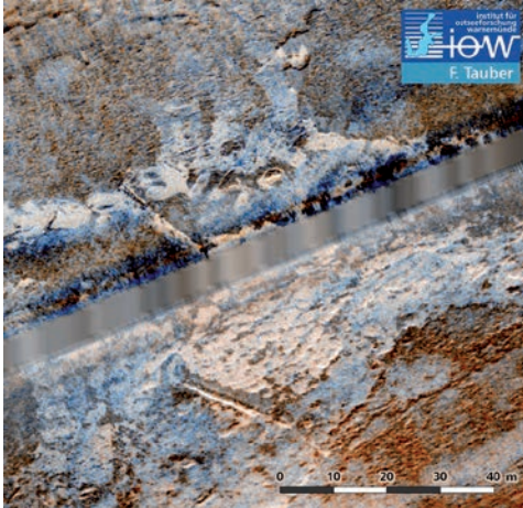
▲ © F.Tauber / IOW. Composite sonar image of the seabed in Wismar Bay, Germany. Detailed sonar recording of large stretches in a preliminary survey can not only reveal individual sites, but can reveal patterns that indicate the presence of eroding Prehistoric landscapes at the bottom surface. Here, a composite sonar image of the sea-bottom in the Wismar bay in the Baltic shows the presence of trees and their roots, the remains of a forest that drowned 6,000 years ago.
