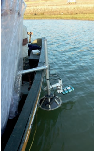
▲ © MMRG, A Knudsen 320 BP Echo-sounder and external receiver, modified by Prof. Lloyd Huff (Center for Coastal Ocean and Mapping, University of New Hampshire), prior to submersion during the Morocco Maritime Survey, Morocco. The echo-sounder, along with its GPS unit, were mounted on a small fishing boat and used to document palaeo-channels and present riverbed bathymetry of the Oued Loukkos as part of the investigation into the location of the ancient port of Lixus, Morocco (October 2010).
