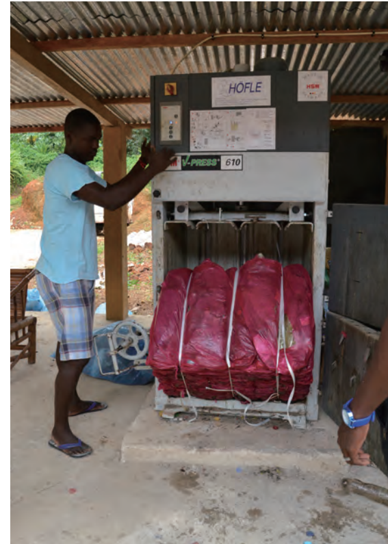
Fig 13. Compacting collected plastic waste to send to recycling
