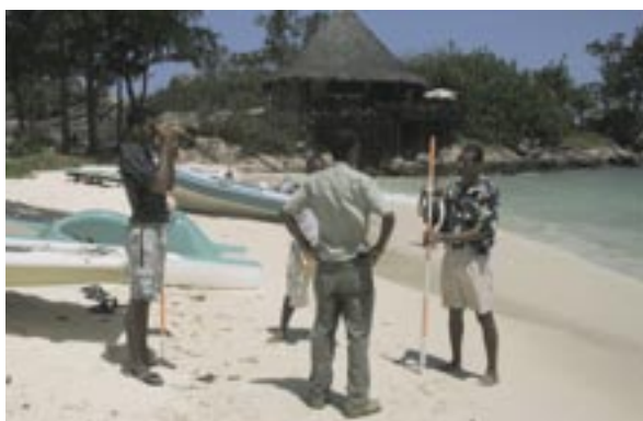
Hotel staff at Lemuria Hotel measuring a beach profile at Anse Petit Kerlan, Seychelles, September 2003
