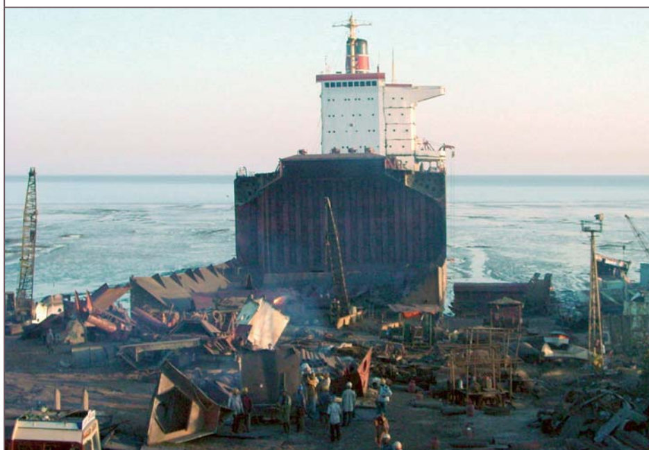
Half-broken ship being prepared to be dragged further onshore
