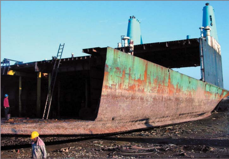
A stripped ship ready for final cutting
