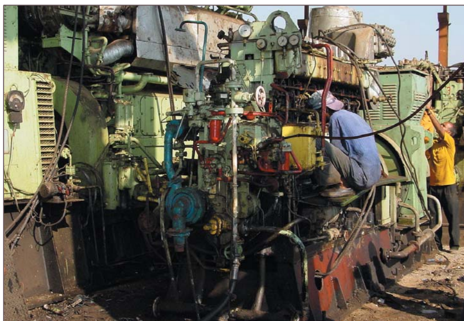
Engine being repaired for re-sale at a khada
