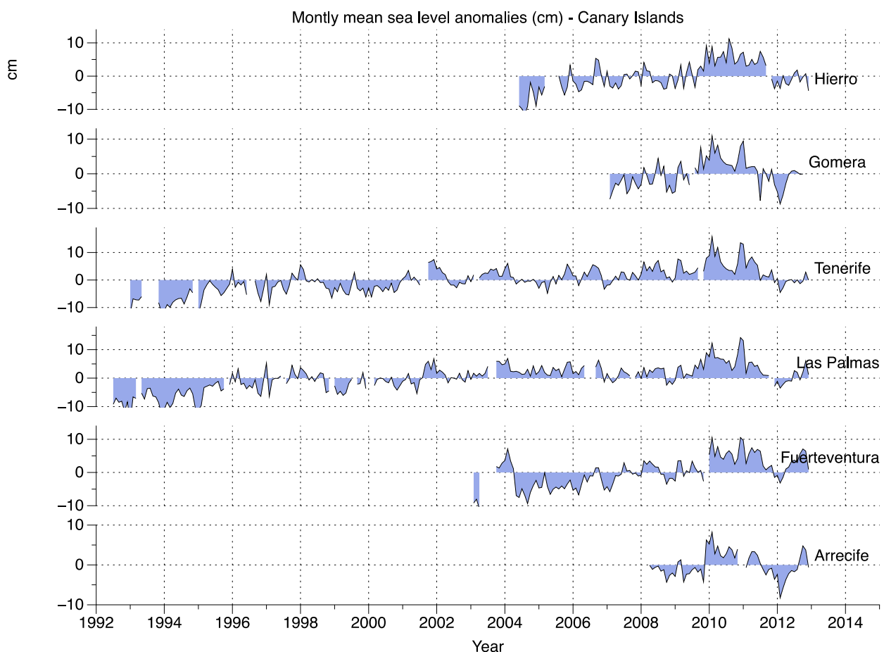
Figure 6.2.2. Monthly mean sea level anomalies at the REDMAR stations in the Canary Islands, since their start date of operation until 2012 (extracted from Pérez-Gómez, 2014).
