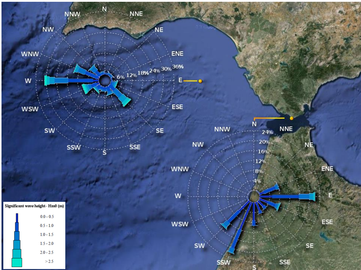
Figure 3.6.5. Wave roses from Golfo de Cádiz (left) and Tarifa (right) buoys (yellow dots)
