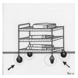
Use a trolley fitted with large rubber wheels. Such wheels keep the manuscripts in a stable position and absorb vibrations.
