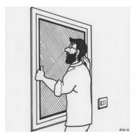
Fit all openings with a grid. Use a grid with sufficiently fine mesh to keep insects out while not restricting airflow.
