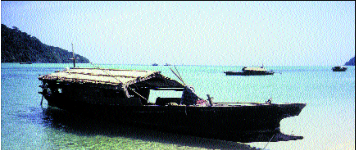
The Moken spend almost half of their life in a 'Kabang', the traditional boat of the Moken. Wooden planks have replaced the Zalacca wood as the preferred material of the gunwale. A bifurcated bow and stern is a distinctive characteristic of the Moken boat.
