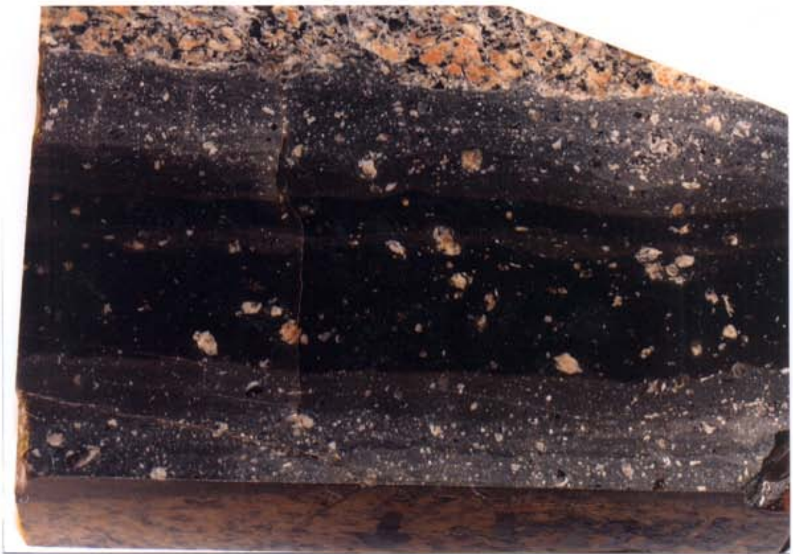
PHOTO 15. PSEUDOTACHYLITE MELT ROCK OCCUPYING THE CENTRE OF A VEIN OF "SHAND"-TYPE, ROCK FLOUR-DERIVED PSEUDOTACHYLITE. THICKNESS OF DARK CENTRE = 20 mm.
