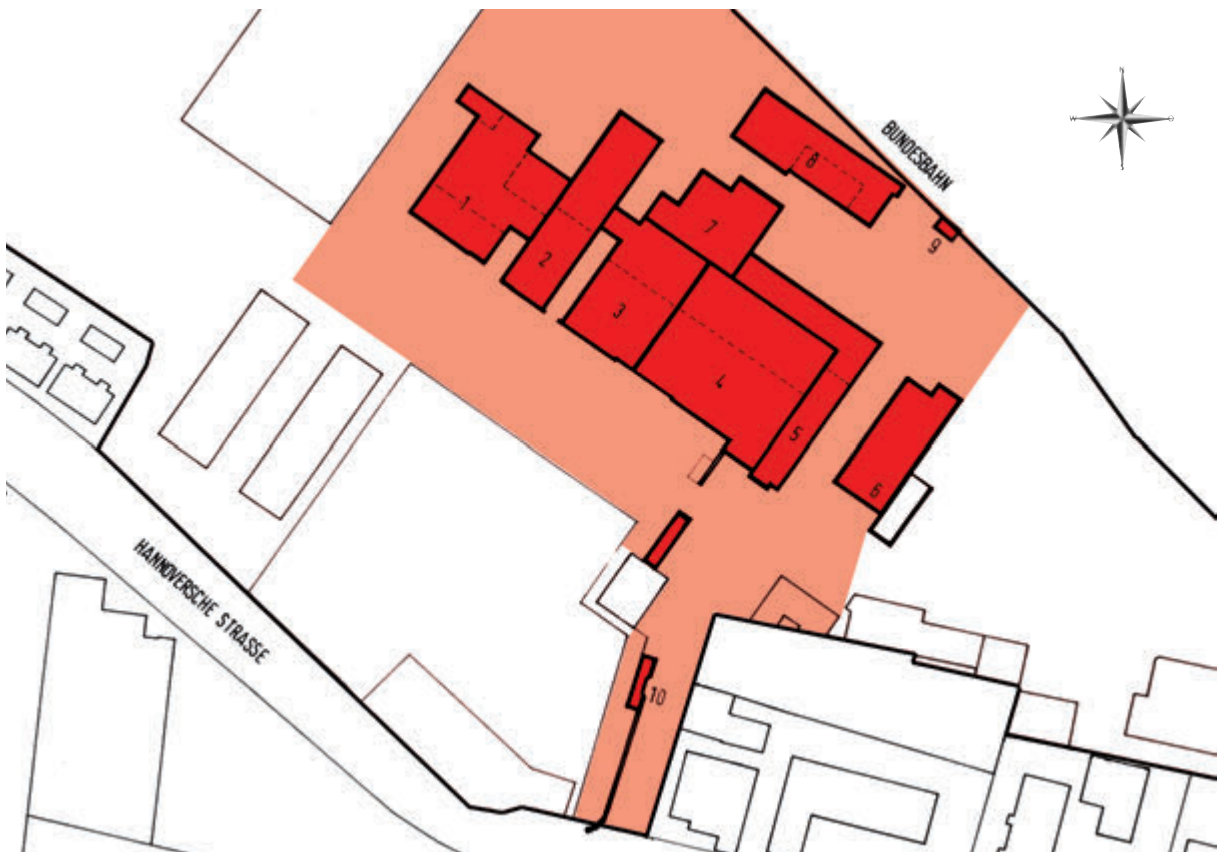
Fig. 9: Floor plan of the Fagus factory, scale 1:2,500 (dark red: main buildings of the Fagus factory; light red: nomination area, section 1: Sawmill, 2: Store house, 3: Drying house, 4: Workroom, 5: Main building, 6: Cutting die department, 7: Engine house, 8: Chip and coal bunker, 9: Rail-car scales, 10: Gatekeeper's house with factory gate and boundary wall)
