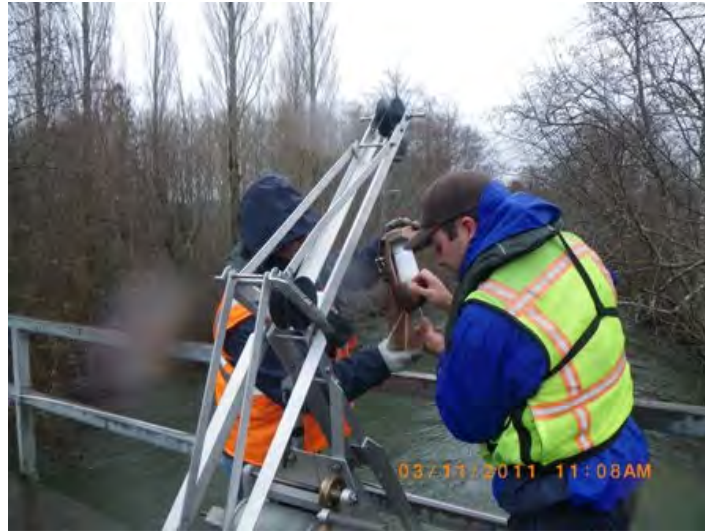
Figure 2: Suspended sediment sampling
