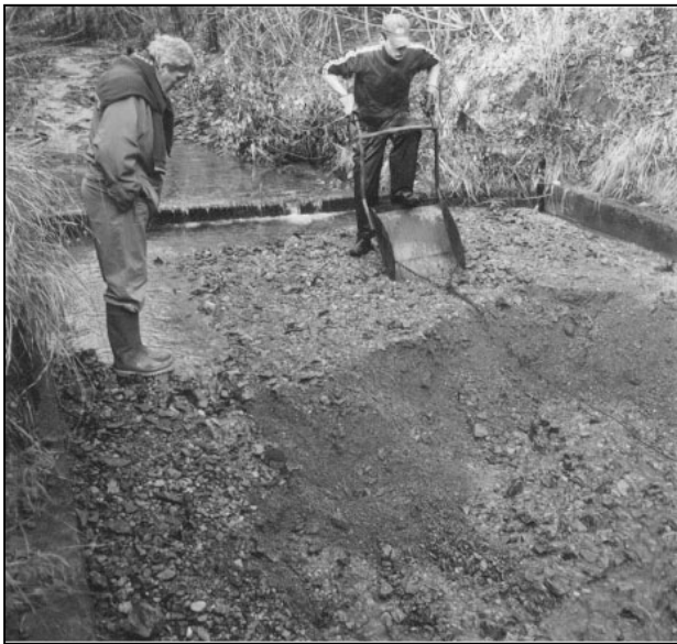
Fig 3. Valle della Gallina experimental basin. On the left: sedimentary pool showing filling condition in November 1992, during the manual cleaning. On the right: grain size zone determined by 27 grain size sample cumulative curves.
