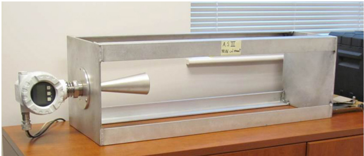
Figure 4.9 An example of a laboratory target used to determine a Sensor Offset (SO) using a range measurement of approximately one metre. The circular flange of the sensor is set flush against the outside surface of the mount, and the distance to the inside surface at the other end of the mount is measured accurately by tape. The distance recorded by the radar is then compared to the tape-measured value giving SO = \text{Tape Range} - \text{Radar Range} . (Photograph R. Heisenrether, NOAA).
