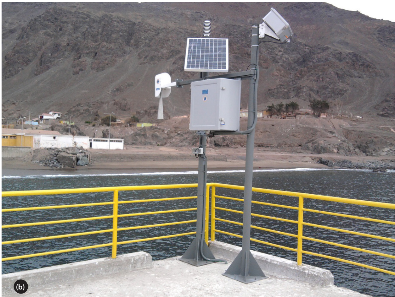
Figure 7.9 (b) A similar BGAN terminal at Taltal, Chile. The antenna (also a T&T Explorer 300) is in the box on the top right of the photograph. (Photograph SHOA).
