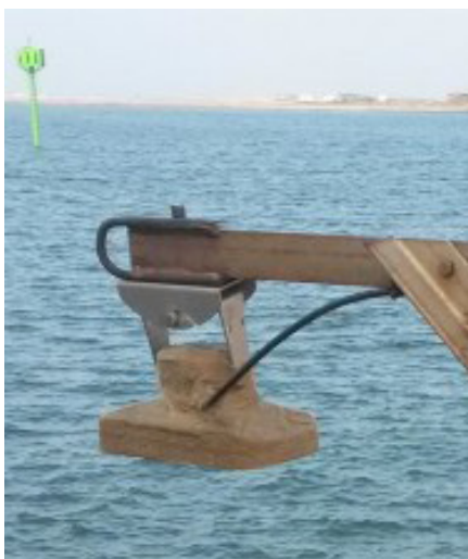
Figure 3. Transducers coated in Denso Tape.
