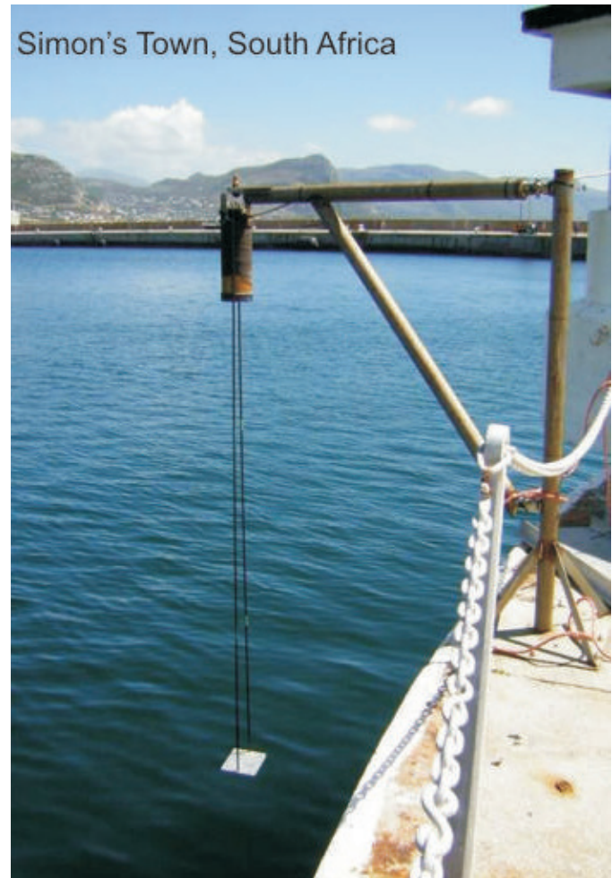
Figure 4.12. Examples of the use of the 'stirrup' target at Luderitz, Namibia and Simon's Town, South Africa. (Photographs Ruth Farre, South African Navy Hydrographic Office).
