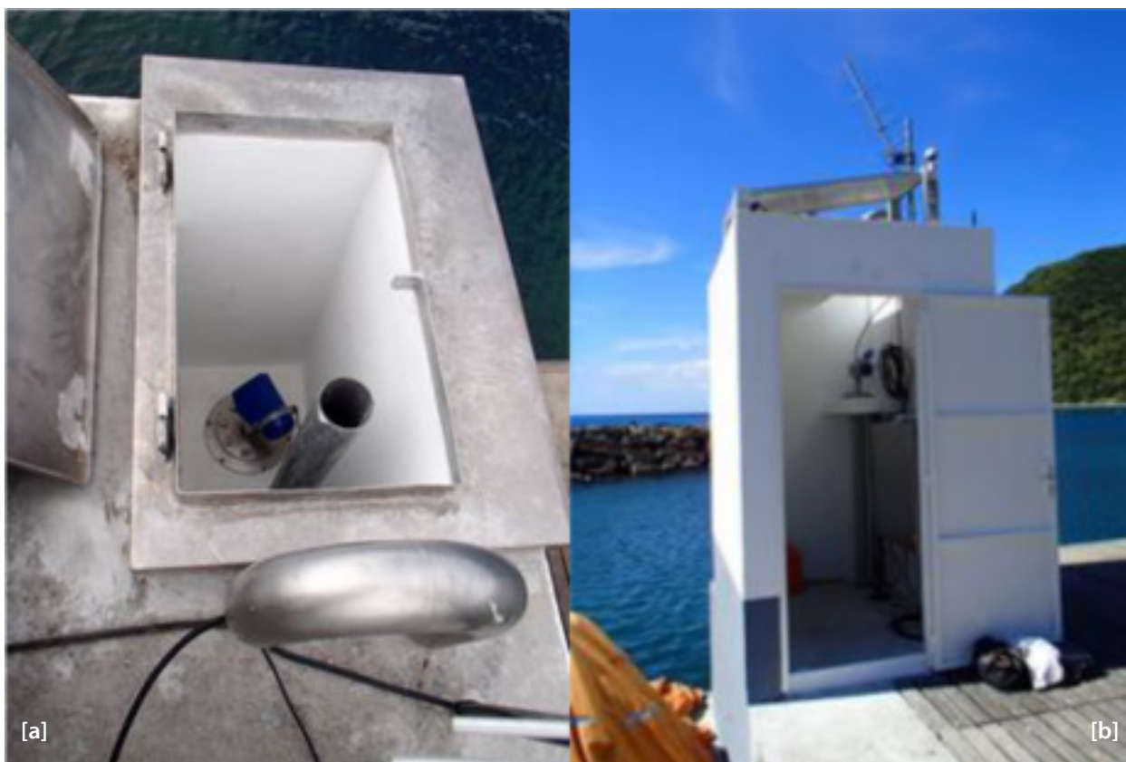
Figure 2 [a] and [b]. Top view [a] and side view [b] of the hatch and housing of the radar sensor in Deshaies, Guadeloupe. The hatch was designed with two functions: first to facilitate the leveling of the radar plate and second to be able to manipulate the stilling well with a crane if necessary (Credit Photo: Sebastien Deroussi, Institut de Physique du Globe de Paris).
