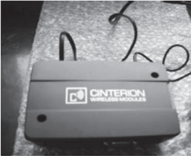
Figure 7.10 A typical GPRS modem as used in Chile.
