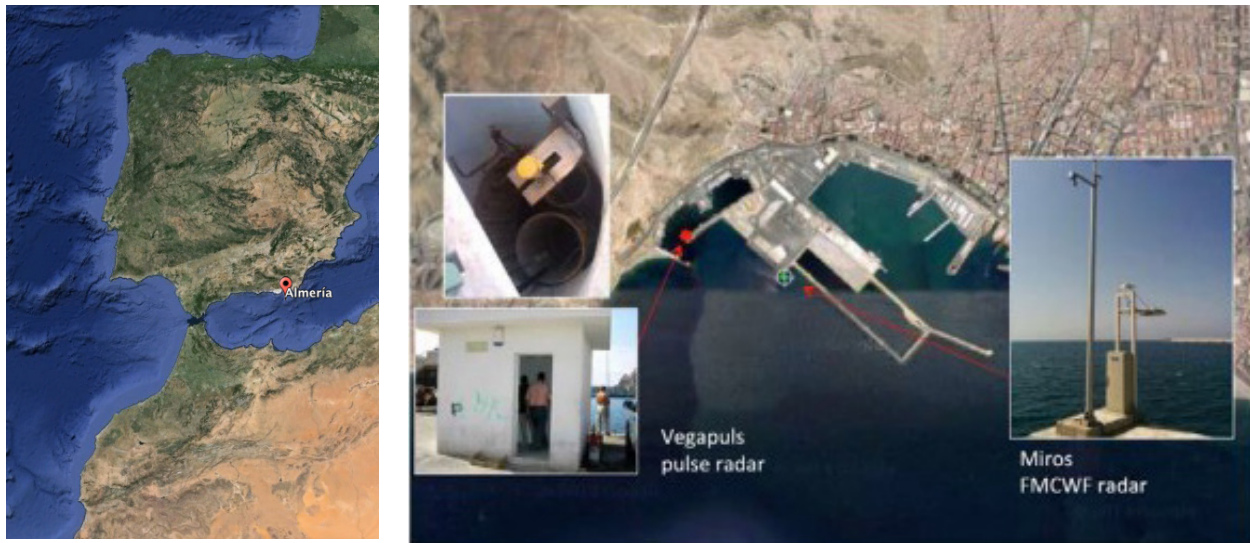
Figure 6. Position of the two radar sensors in Almería: VegaPuls (pulse radar) from IGN and Miros FMCWF radar from PdE (REDMAR).
