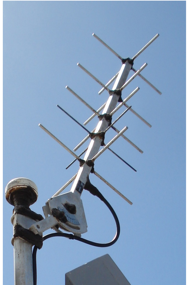
Figure 7.8 A GOES Yagi antenna. The small hemisphere on the top of the support post is a GPS antenna for time control. (Photograph NOC).
