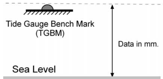
Figure 53. Generic figure about datum information. The data reference is the Tide Gauge Bench Mark (TGBM). Source: Área de Geodesia, IGN
