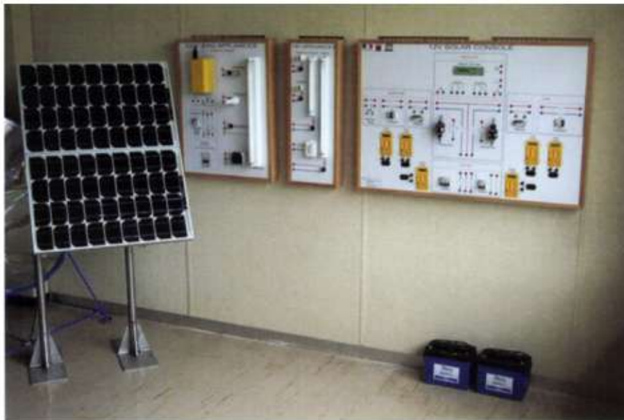
Training platform for solar lighting systems (UNESCO)
