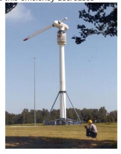
how NASA tested a one-bladed rotor configuration. (Photo by NASA Glenn Research Center)
