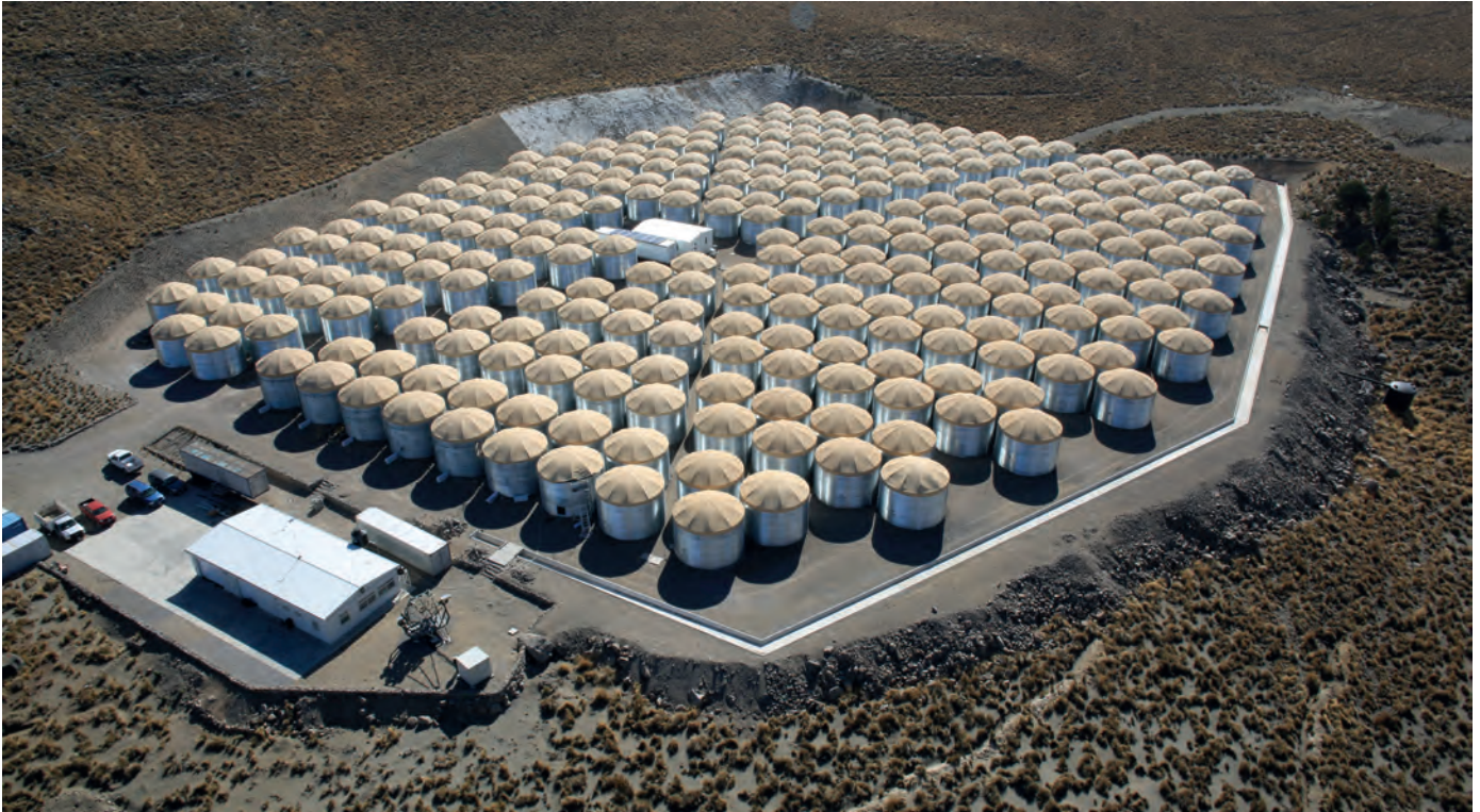
Figure 2. Drone view of the HAWC Gamma Ray Observatory on its inauguration, 20 March 2015. The array is approximately 150 m on each side, with a single detector 7.2 m in diameter. © INAOE.
