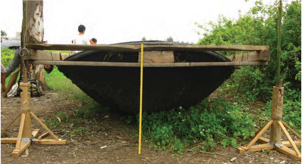
Boat Tuong 14 with stands along which measure tapes and references can be strongly fixed. Mr. Toan Huyen's boat yard, Huong Hoc village, Quang Ninh province. © Charlotte Minh-Hà Pham
