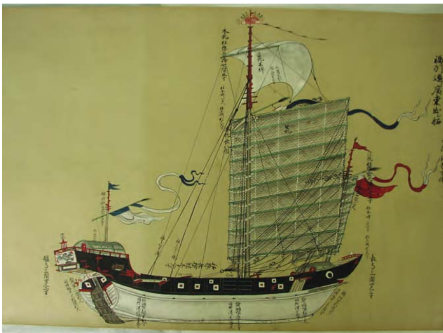
A fuzhou ship is typically a Southern Chinese ship-building tradition. It is possible to recognize the bamboo battened sails, a clear hanging axial rudder and a keel. This ship also figures on the eighteenth century picture scroll 'Tosen no Zu' (Matsura Historical Museum). © Matsura Historical Museum/Jun Kimura
