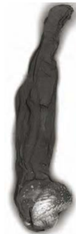
TOP: Wood from the Avondster ship (Galle, Sri Lanka) severely attacked by the shipworm. © MAU
