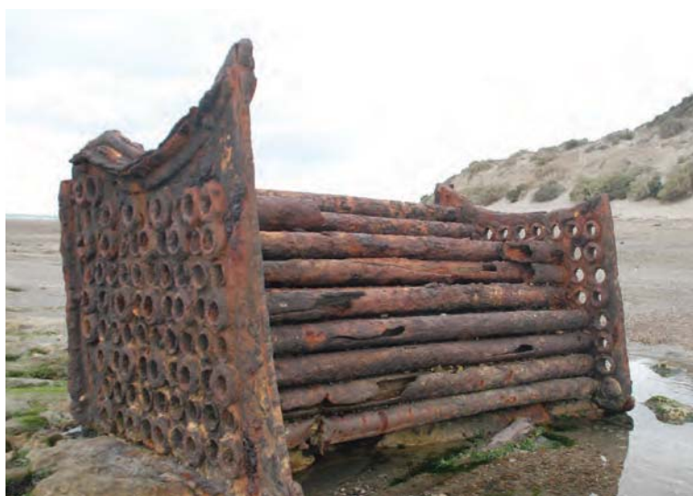
A section showing the steam pipes from a broken boiler. © Christopher J. Underwood
