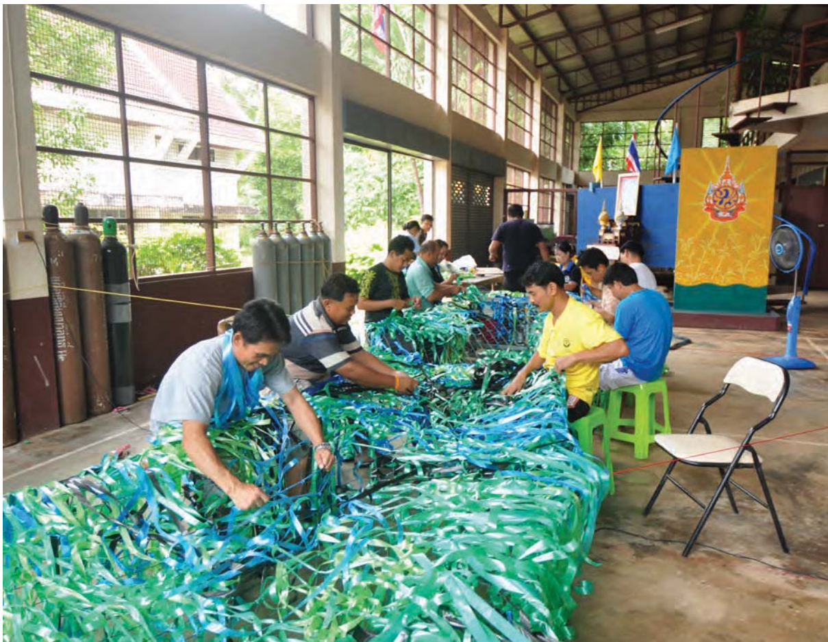
Artificial seagrass can be bought or made by hand. Here, the UAD in Chanthaburi are making their own seagrass by assembling large (approximately 1 metre) fronds on fishing nets. © UAD, Thailand
