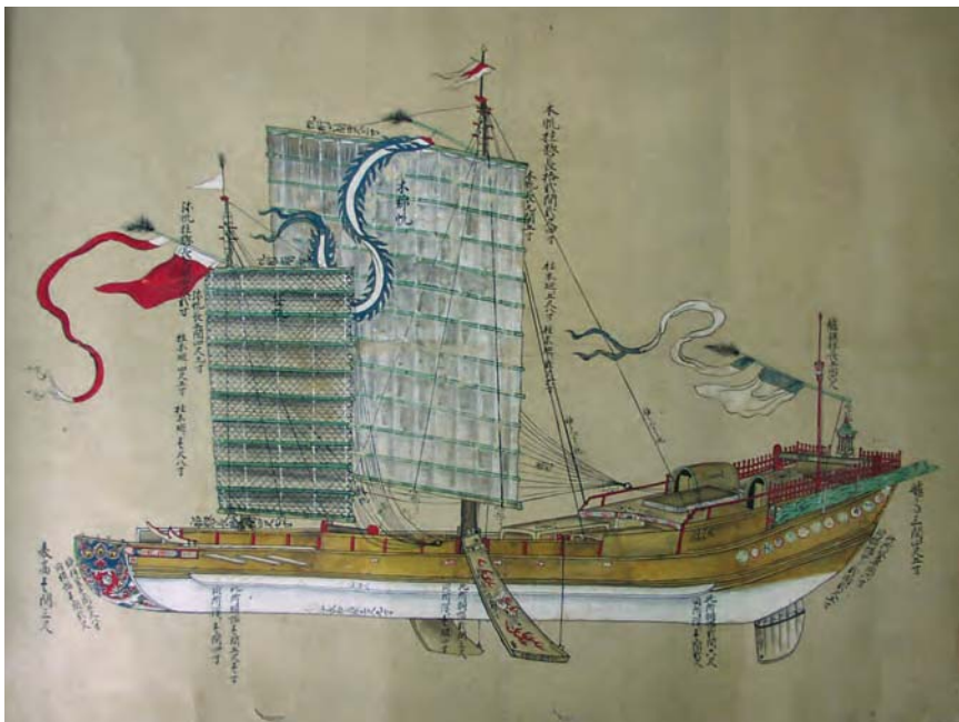
A nanjing or sand ship has a flat bottom that allows it to theoretically be beached or to travel in river channels. On this Chinese merchant ship depicted on the eighteenth century picture scroll 'Tosen no Zu' (Matsura Historical Museum), it is possible to clearly see the flat transom and the leeboards. This type of ship belongs to a Northern type of Chinese boat building tradition. © Matsura Historical Museum/Jun Kimura
