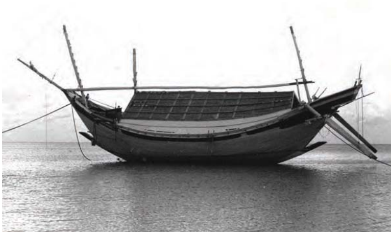
A large janggolan with the sailing rig removed, laid up for the monsoon. In Madura, janggolans are dedicated to freight work, usually carrying a salt cargo. © Kurt Stenross
