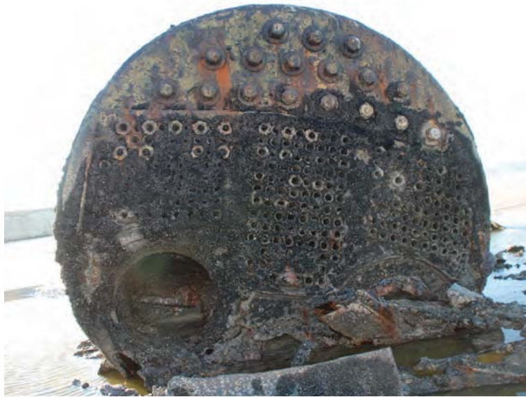
ABOVE AND BELOW: Front and starboard side views of a steam (Scotch) boiler. © Christopher J. Underwood
