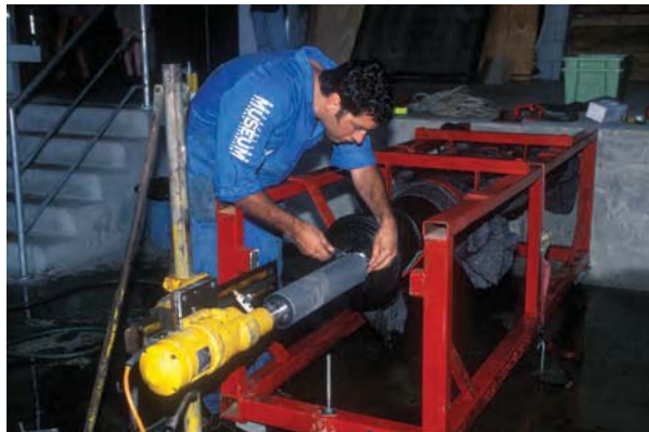
Andrew Viduka working on boring out the barrel of a six pounder gun from HMS Pandora prior to electrolysis treatment. © Queensland Museum
