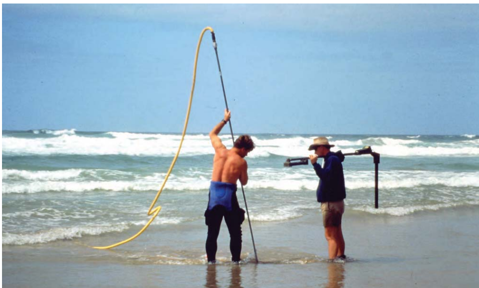
Water probe in operation on the Hive site, Australia. © Andrew J. Viduka
