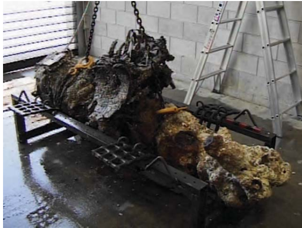
Concreted six pounder gun from HMS Pandora on a treatment cradle. © Queensland Museum
