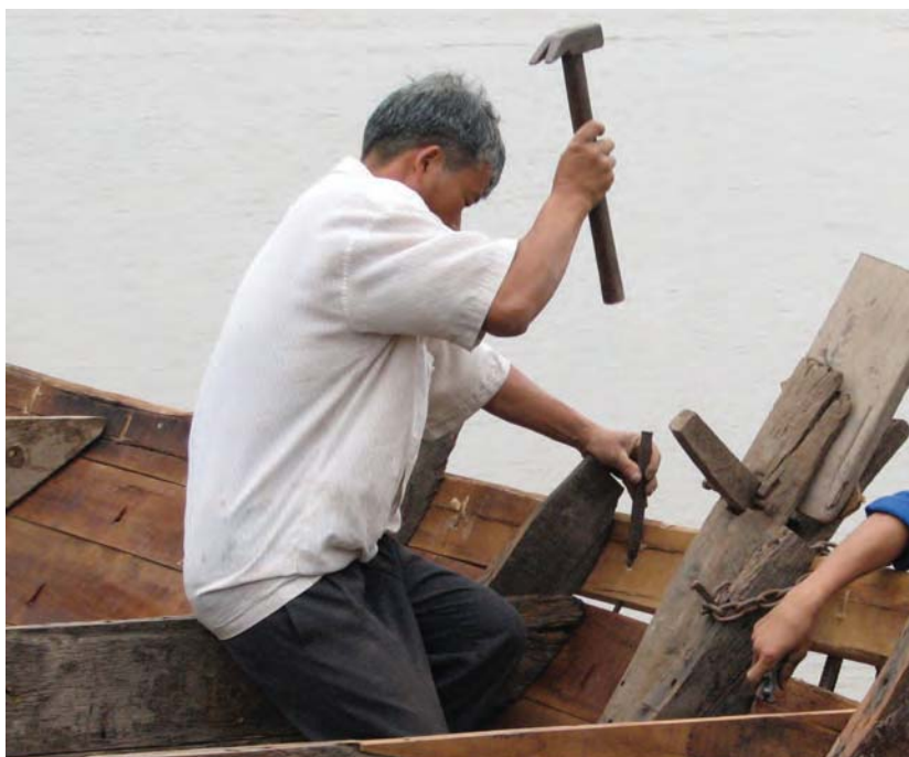
Boat building in Northern Viet Nam, demonstrating the Chinese tradition of using iron nails. © Colin Palmer
