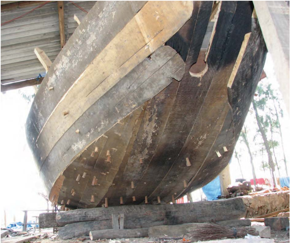
Boat building in Southern Viet Nam, demonstrating the South-East Asian tradition of using wooden pegs. © Colin Palmer
