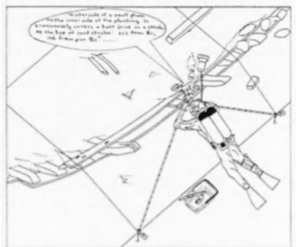
Below, trilateration measurements being carried out on the Medemblik wreck. All information was spoken into a tape recorder.
